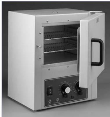
A compact embedding oven ideally suited to polymerisation of resins in a fume cupboard. The temperature is controlled by a thermostat fitted to a calibrated scale with a locking device. There is a hole in the top of the oven for a thermometer. The oven contains two removable shelves.
