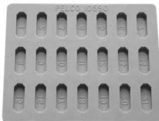
Blue silicone rubber mould with 21 numbered cavities with double pre-trimmed ends.
