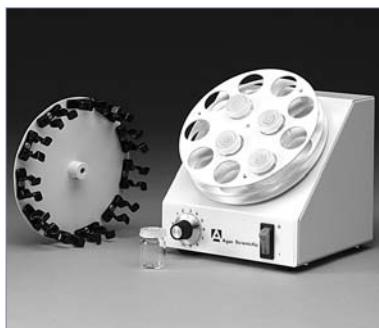
This fixed tilt rotator holds up to 12 glass vials. It is designed to improve penetration of fixatives and resins into biological tissues prior to polymerisation. It has continuously variable speed in the range of 2 to 26 rpm. The compact size allows the rotator to be used in a refrigerator or incubator, as well as on the bench. Additional discs are also available.
