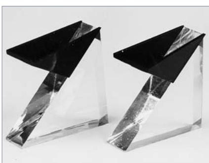
These are disposable, moulded plastic troughs for fitting to glass microtome knives. They provide a reproducible and clean trough which is quickly and easily attached to the glass knife with wax. The Trufs have ample capacity for large ribbons of sections.
