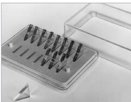
These dust free containers have silicone rubber mats with numbered recesses for 16 knives. Two sizes are available to hold 25 x 25 x 6 - 7 mm or 25 x 25 x 8 mm knives.
