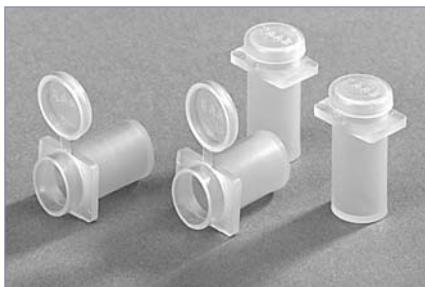
Flat ended capsules, 8 mm in diameter, available in polyethylene for embedding at temperatures up to 75 °C, or polypropylene for embedding at temperatures up to 100 °C.
