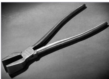
Substantial pliers designed to give a good break. They have an end mark on the jaws to locate the break line.
