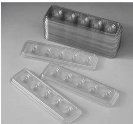
These are disposable, transparent plastic moulds. Each mould has five impressions. Suitable for use with plastic embedding stubs (**G3552**), to produce ready mounted blocks for direct attachment to a microtome.
