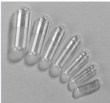
Pure gelatin capsules, providing a convenient and economical means of producing resin blocks for sectioning. They are easy to remove from the resin block prior to sectioning.
