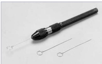
Platinum loop in a pin vice, providing a readily cleanable loop.
