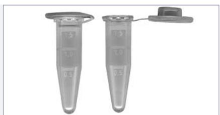
Manufactured from high quality coloured polypropylene that withstands forces up to x30,000G. Graduated 0.1 and 0.25 ml. Available in red, yellow, blue, green and orange. 100 of each make a pack of 500.
