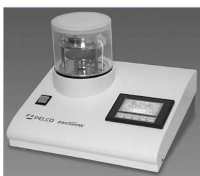
This is a compact, stand alone, easy to use discharge cleaning system primarily designed for surface modification of TEM support films. The system supports both hydrophilic and hydrophobic treatments for either a negative or positive charge and includes two separately controlled gas inlets.
