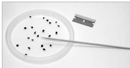
100 mm diameter dishes for trimming, cutting and specimen preparation.
