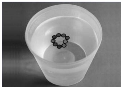
Static free, graduated 30 ml polypropylene cups, ideal for preparing water for glass or diamond knife troughs. They ensure distilled water is static free, so that serial sections will not move around the trough.
