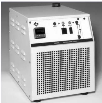
A water chiller/thermocirculator offering accurate temperature control from -5 to 60 °C. It can be used to pre-cool the chamber prior to specimen loading then increase the temperature to the critical point. It has a 400 W heater, and is fitted with an over temperature cut out. Dimensions: 370 x 320 x 460 mm. Weight: 40 kg.
