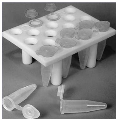
This holder made from Teflon® is designed to hold up to 18 conventional polyethylene microcentrifuge tubes firmly in the water bath during curing.
