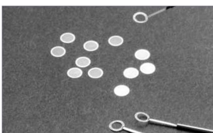
Using this loop, thin sections can be transferred easily from microtome boats to grids with a minimum of creasing or folding.
