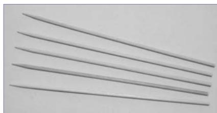
Bamboo splints offer a simple method for holding tissues for mincing or cutting. Pointed on one end. 150 mm long.
