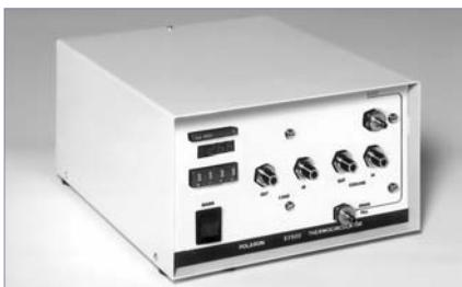
500 W water heater/circulator with a working range from ambient to 60 °C, allowing the temperature of circulating fluid to be pre-set. It can be connected directly to the water jacket inlet/outlet of critical point dryers, and is fitted with an over temperature cut out.
