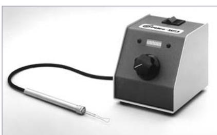
This heat pen helps to reduce compression in plastic embedded sections. Suitable for replacing solvent vapour methods. Variable temperature control with coloured light bars which flash to indicate temperature and warn the operator of the hot filament. The filament and holder can be clamped onto the back of the housing when not in use.
