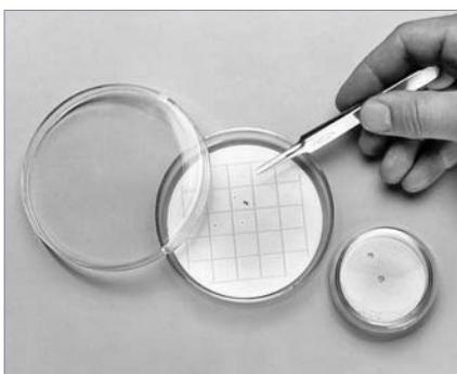
Grip-a-grid storage disc offering secure storage of grids in a Petri dish. Each disc is marked with numbered squares to allow easy identification of specimens, and prevents grids being easily knocked out of position. Grip-a-grid discs are easy to clean, and are available to fit 50 and 90 mm round and square Petri dishes.
