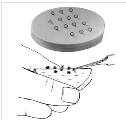
Flexible silicone pad designed for staining grids, as well as holding tabbed grids, Omniprobe grids and samples. It has 18 slots which support grids securely, even when the pad is flexed. When the pad is laid flat the grids stand vertically allowing the surface tension of the droplets of stain to cover both sides of the grid.
