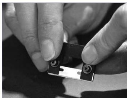
A simple device designed to safely hold unbacked single edge razor blades. Easy to reload.
