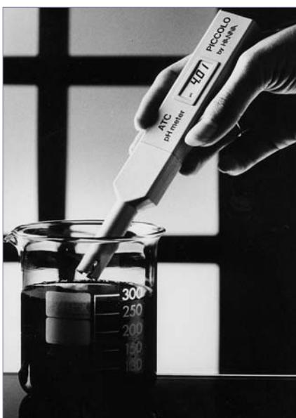
An easy to use, battery operated pH meter, offering bench type accuracy with automatic temperature compensation. It can be used for stirring while the readings are being taken. The electrode is replaceable. The four 1.4 V batteries give 1000 hours of use. It is supplied complete with electrode, pH 4 and pH 7 buffer solutions and a calibration adjustment screwdriver, in an ABS carrying case.
