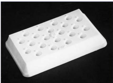
This numbered rack for 22 BEEM 00 capsules holds them upright for filling and curing. A vacuum relief hole in the bottom of each depression permits light transmission for examination of the blocks. This holder is also suitable for gelatin capsules.
